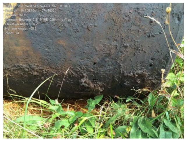
28. Pitting on removed underground storage tank
